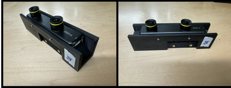
Figure 14: Left camera housing installation.
