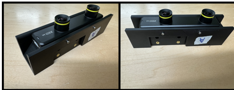
Figure 13: Right camera housing installation.
