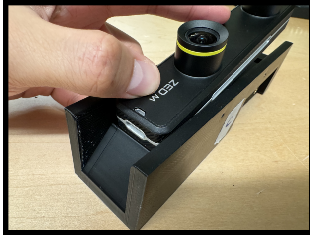
Figure 12: The edge containing the port on the camera should always be aligned with the edge of the ramp of the camera housing. Install each camera as shown here.
